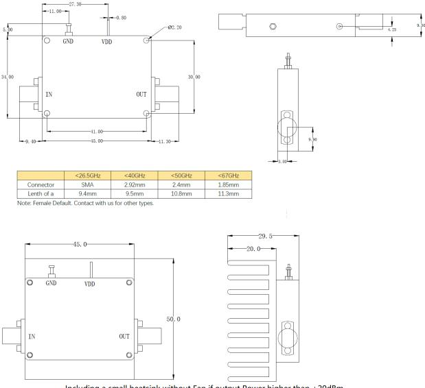
Including a small heatsink without Fan if output Power higher than +20dBm. Customers can removed it or use their own heatsink according to actual situation.
